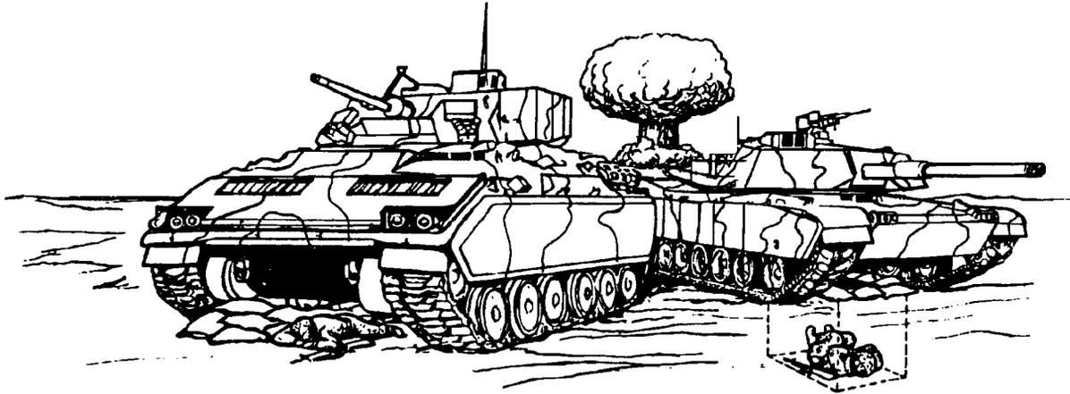
Figure 4-4. Tracked vehicle as expedient overhead cover.
