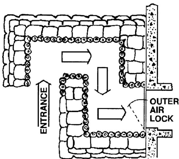
Figure 4-12. Protection from blast flow into shelters.
