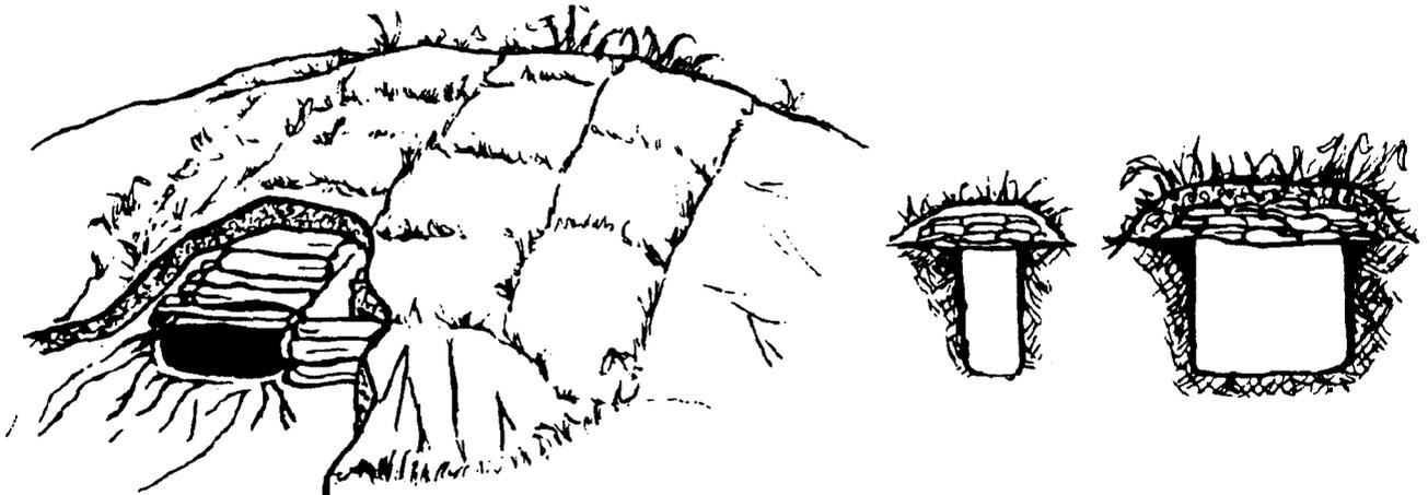
Figure 4-6. Sandbags protected with sod and earth cover.
