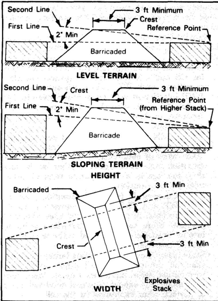
Figure 2-3. Barricade Dimensions Between Explosives Stacks.
