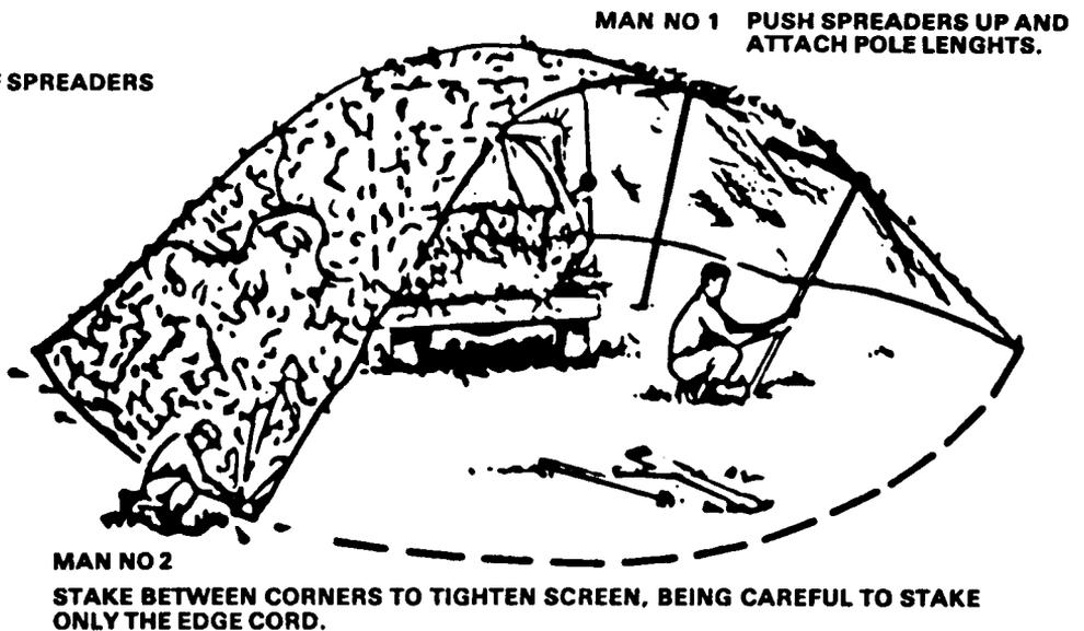
FIGURE 20-3. Procedures for Erecting a Two-Module Camouflage Screen System (Continued).
