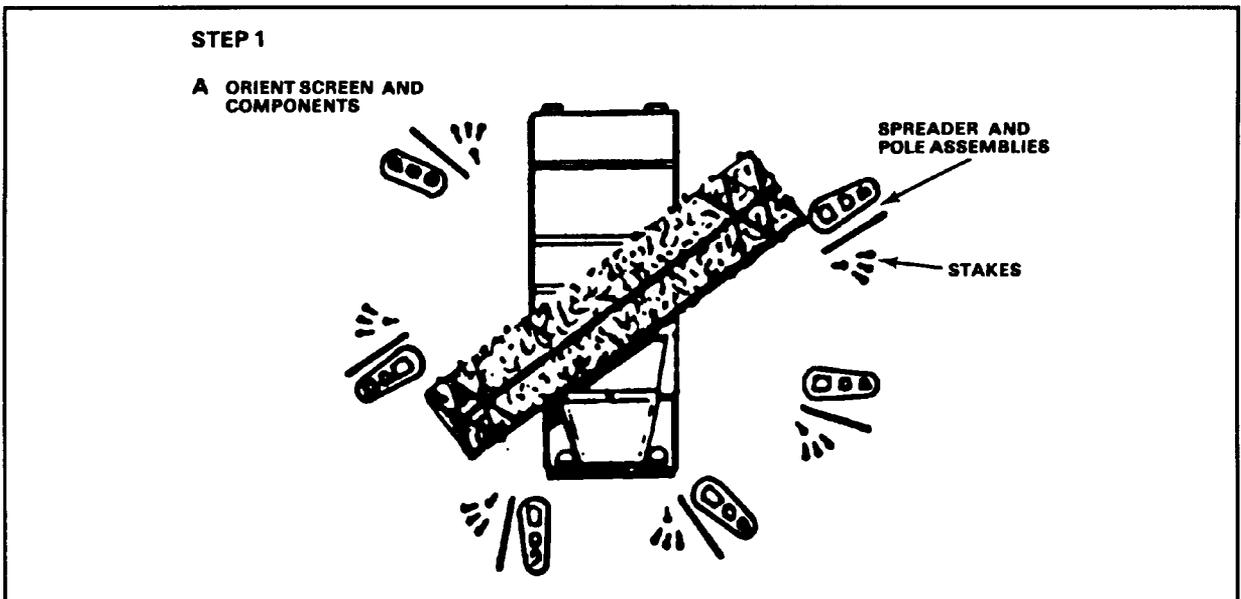
FIGURE 20-3. Procedures for Erecting a Two-Module Camouflage Screen System.
