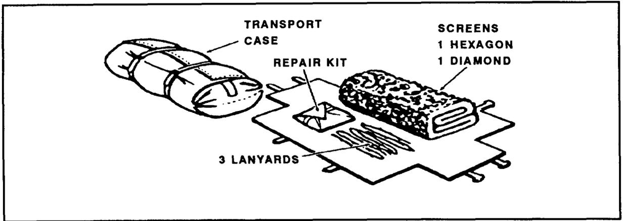
FIGURE 20-2. Screen Transport and Storage Case (With Components).
