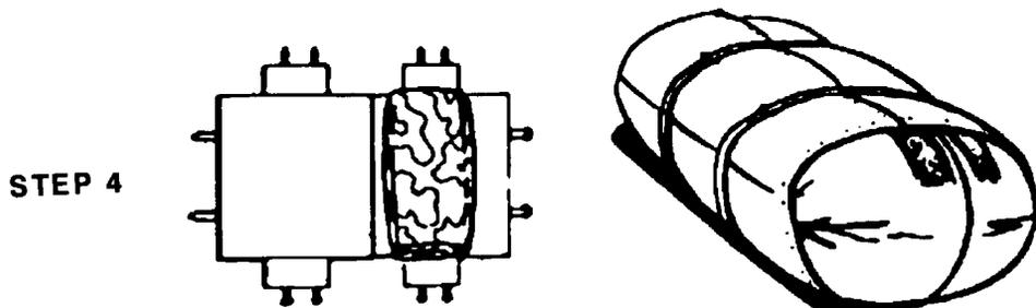
FIGURE 20-5. Method of Folding Screens for Storage.
