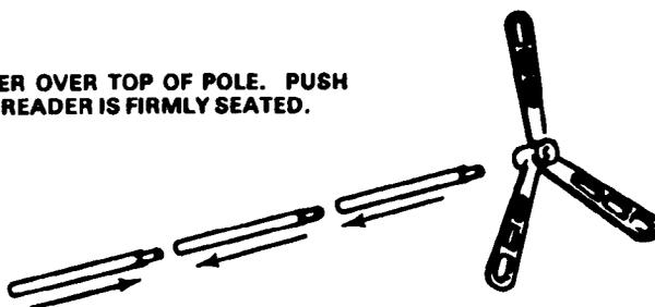
**C TO INSTALL SPREADERS, LOOSEN TOP NUT.**
