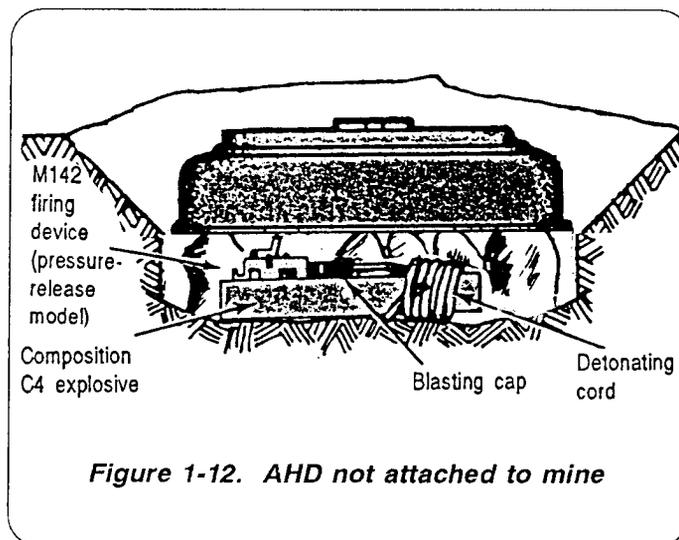
Figure 1-12. AHD not attached to mine
