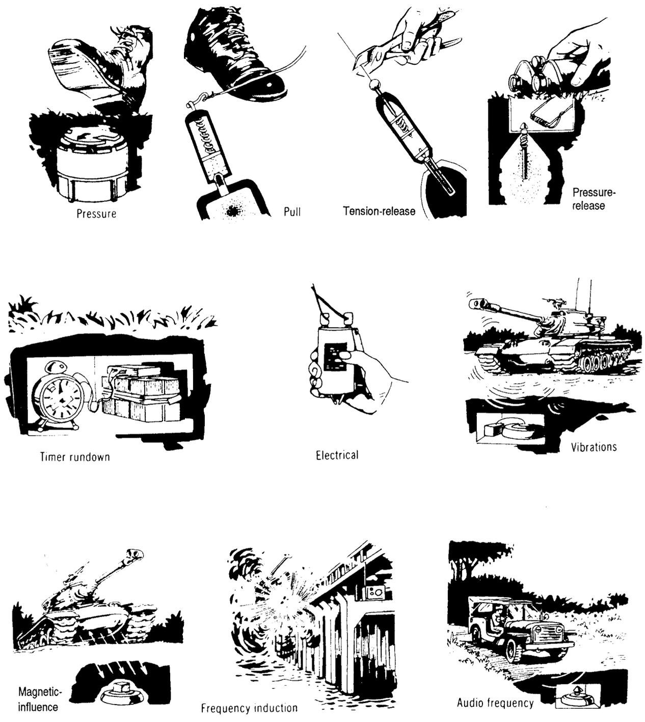
Figure 1-2. Methods of actuating mines
