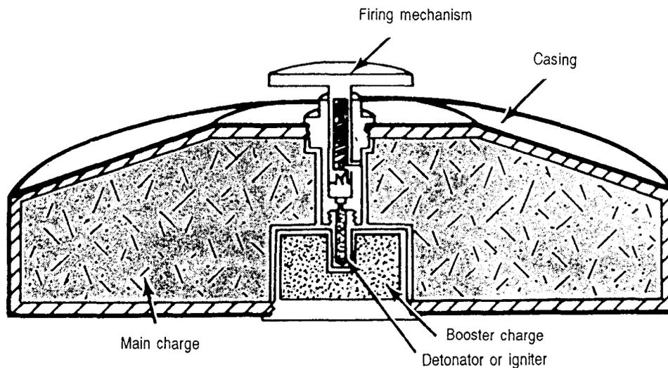
Figure 1-1. Mine components
