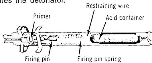
**Friction.** The initiating action ignites substances inside the fuze by friction. The flame fires the detonator.
