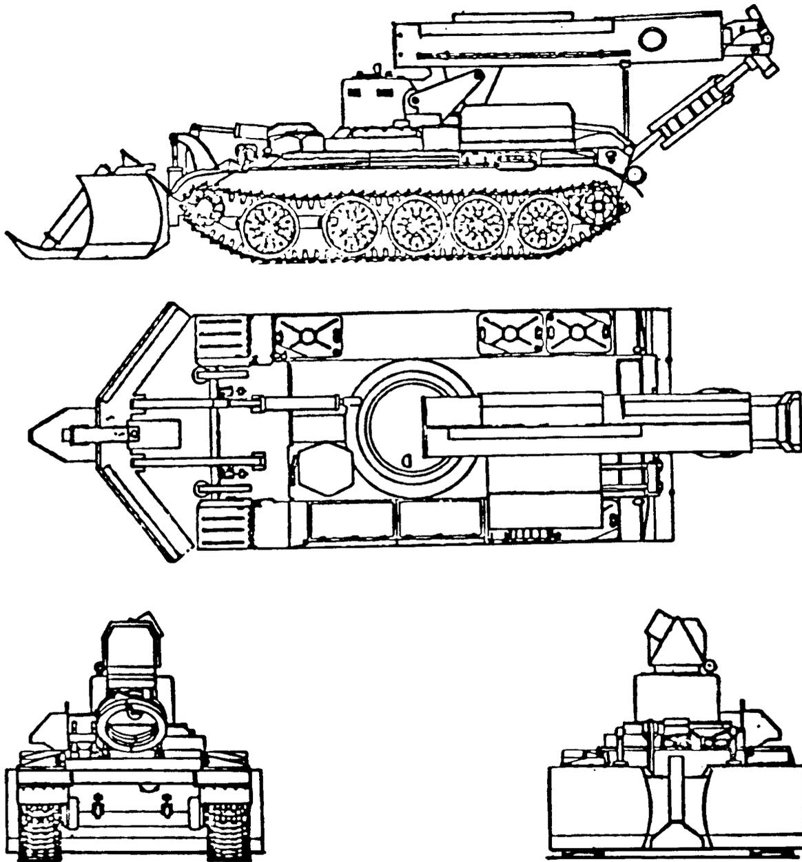
Figure C-11. IMR armored engineer tractor
