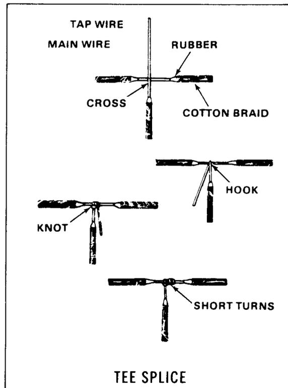
Fixture. Used to join a small wire to a large one, or to join a thin wire to a thick one.
