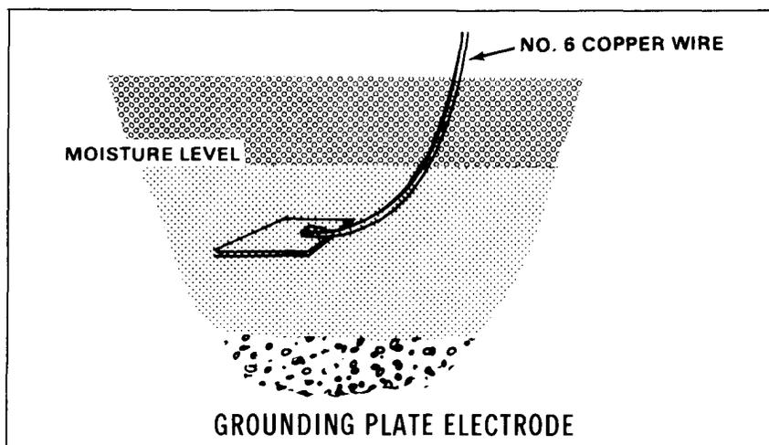
Attach the grounding system with No 6 American wire gage or a larger cable. Connect one end of the cable to the grounding terminal of the generator set. Tighten the nut securely, as described in the appropriate technical manual. Connect the other end of the cable to the grounding electrode with a special grounding clamp.
