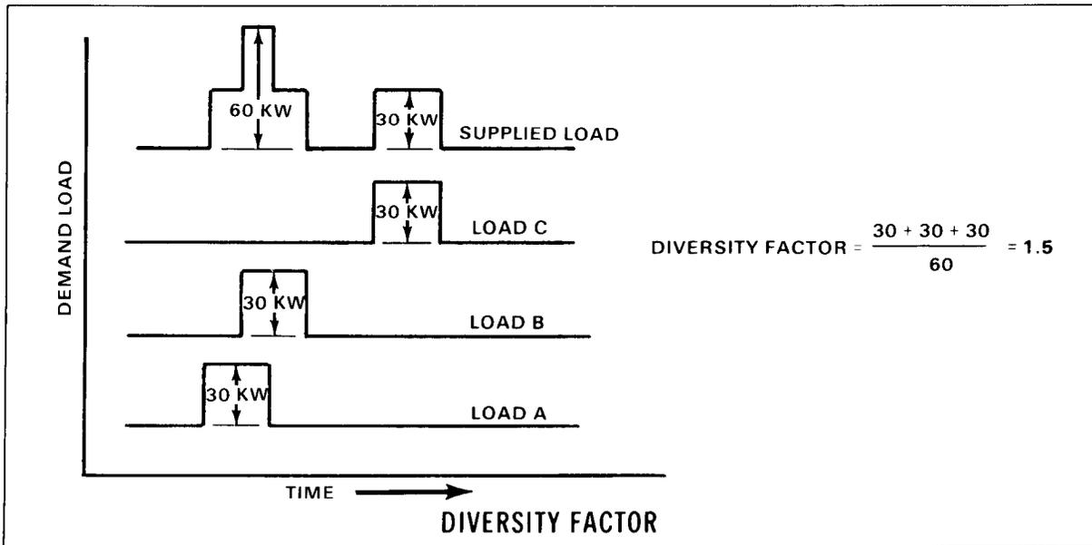
Demand and diversity factors are used in planning the design of electrical facilities. They are used to determine the type and size of generator sets required for a field unit. Demand factors also are used to rearrange existing facilities. For example, additional equipment may greatly increase the connected load for a structure, but it may or may not require a change to the serving generator set.
