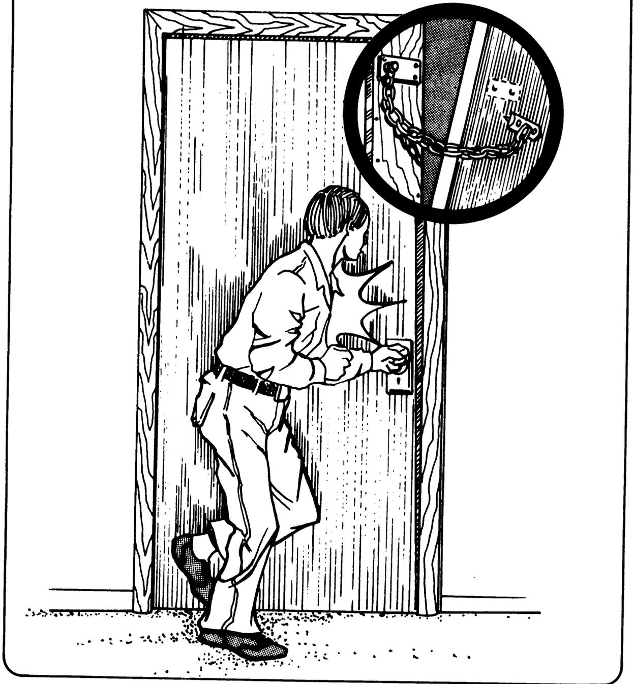
*Figure 66—Most chain latches require little effort to neutralize.*
