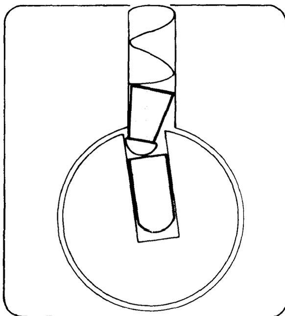
**Figure 62—Example of mushroom tumbler action during picking.**
