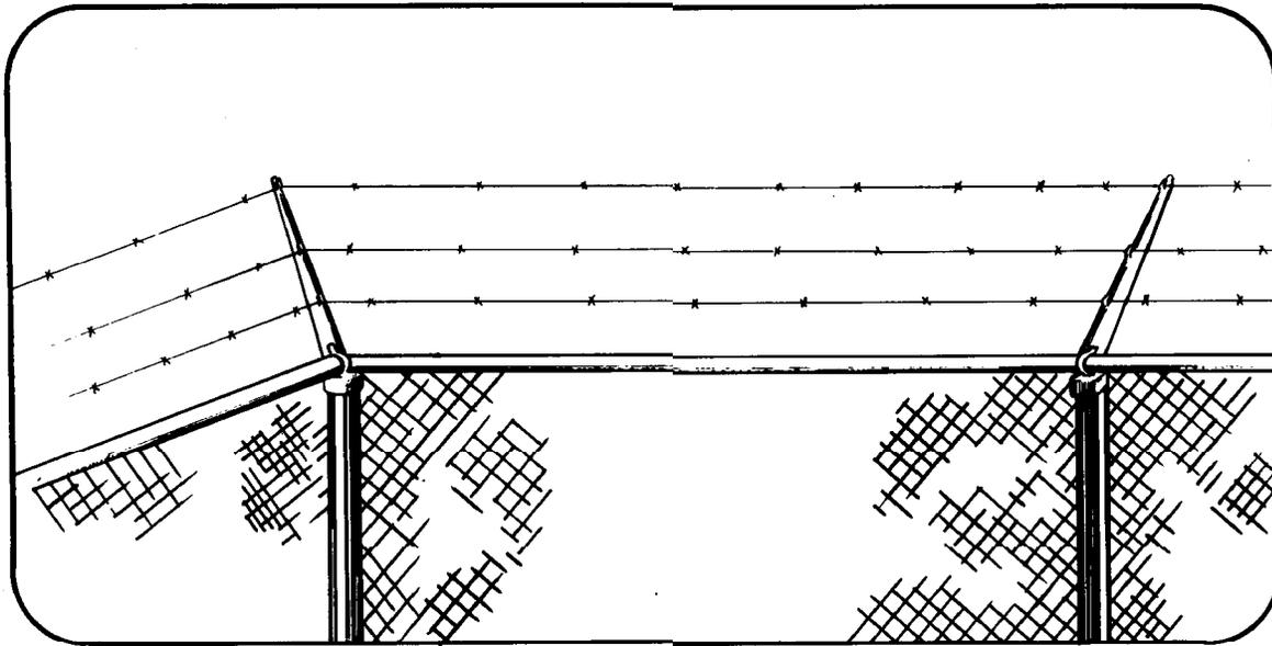
*Figure 14—Supporting arms on top guard point outward.*
