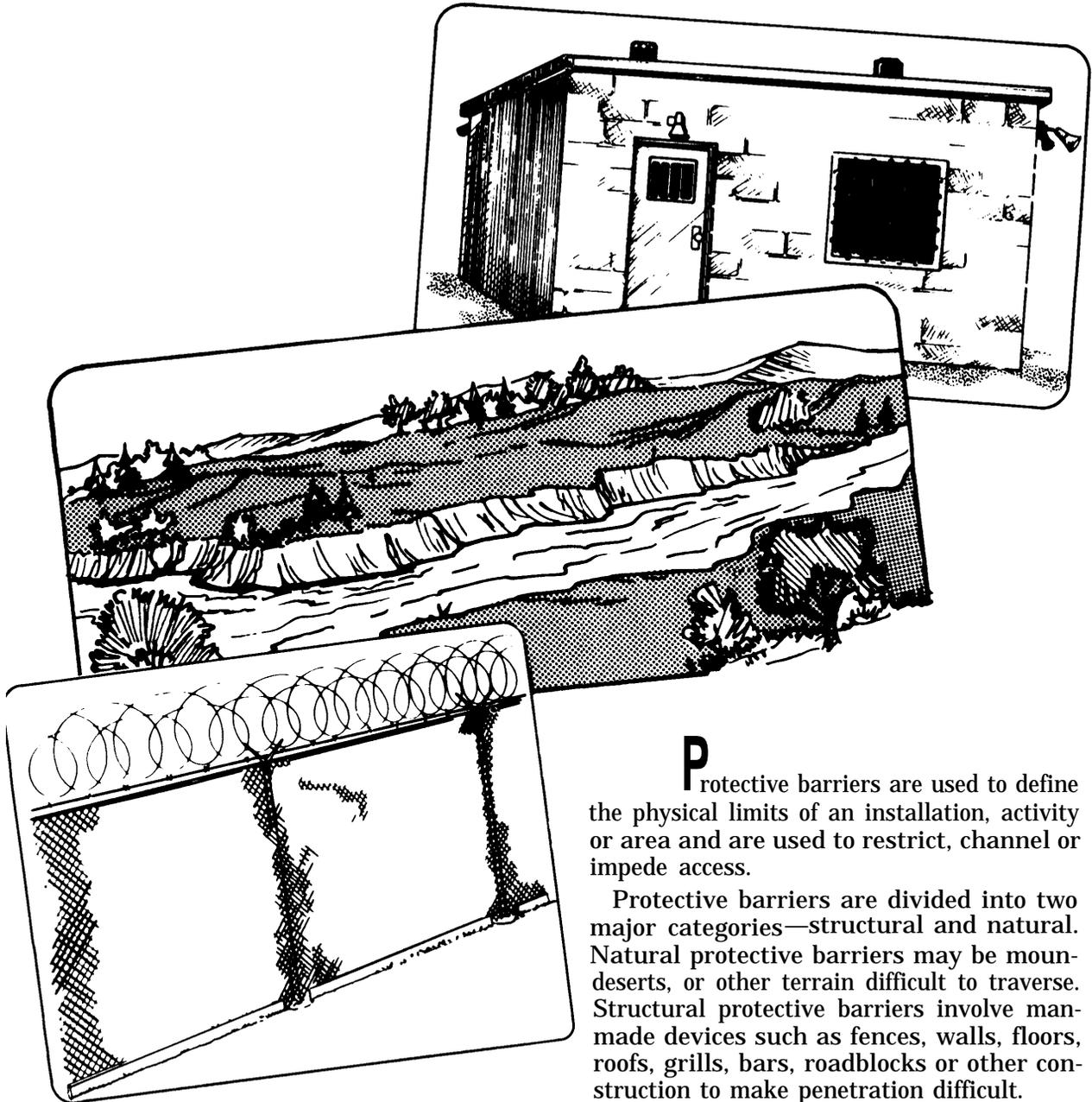
**P**rotective barriers are used to define the physical limits of an installation, activity or area and are used to restrict, channel or impede access.
