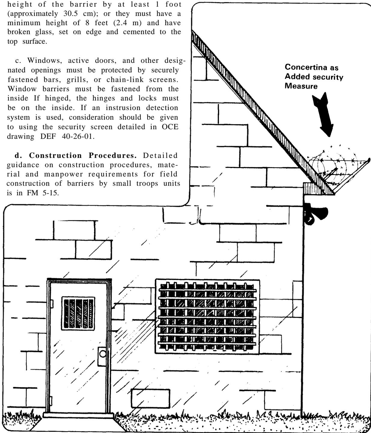
Figure 17 - Sample of top guard on roof.
