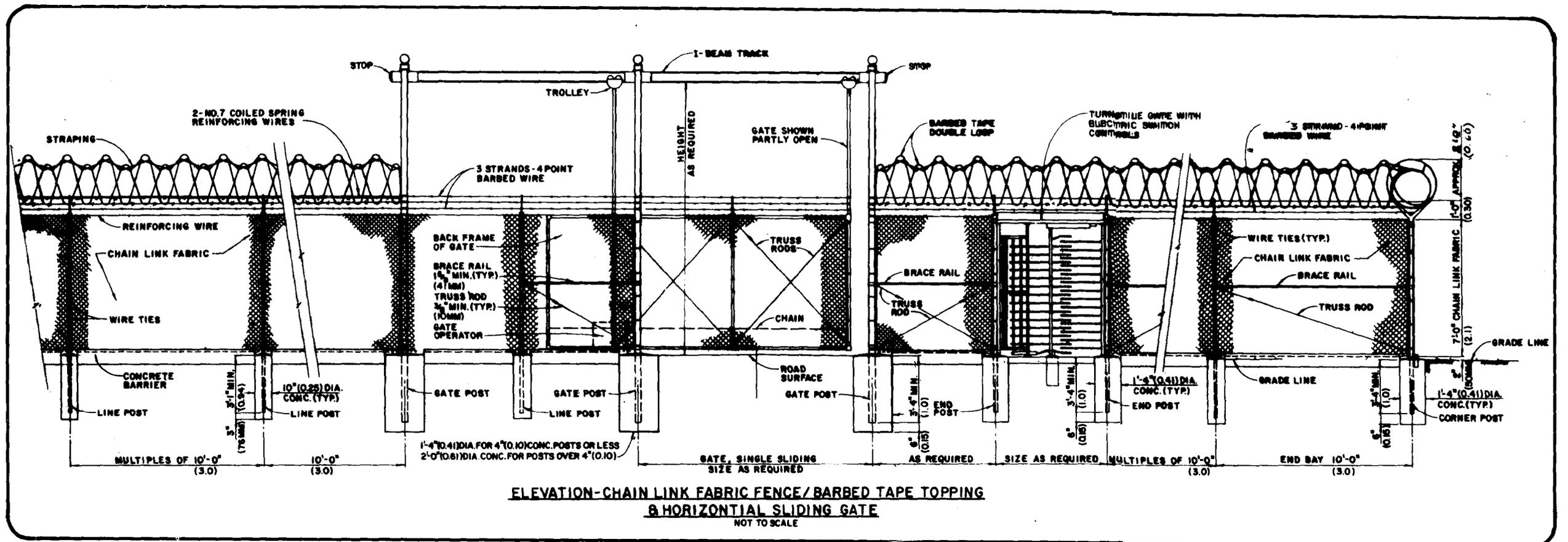
Figure 11—OCE drawing 40-16-10 of chain link fence construction.
