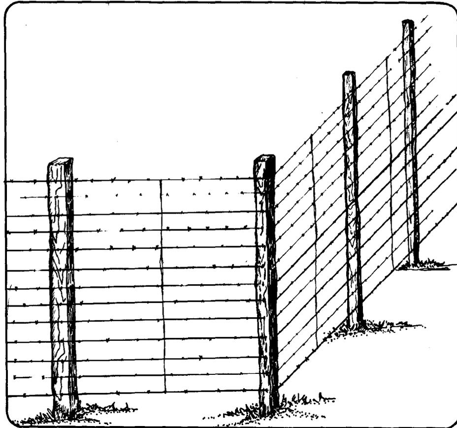
Figure 12—Example of properly constructed barbed wire fence.
