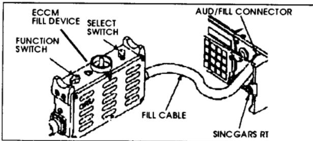
**Figure 4-12. Loading FH data fill.**
