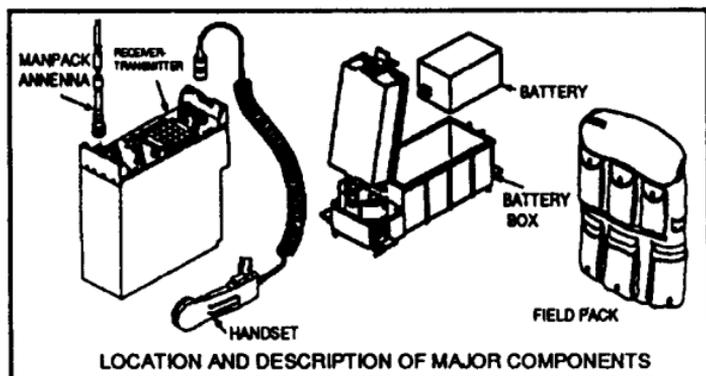
Figure 4-7. Radio set, AN/PRC-119.
