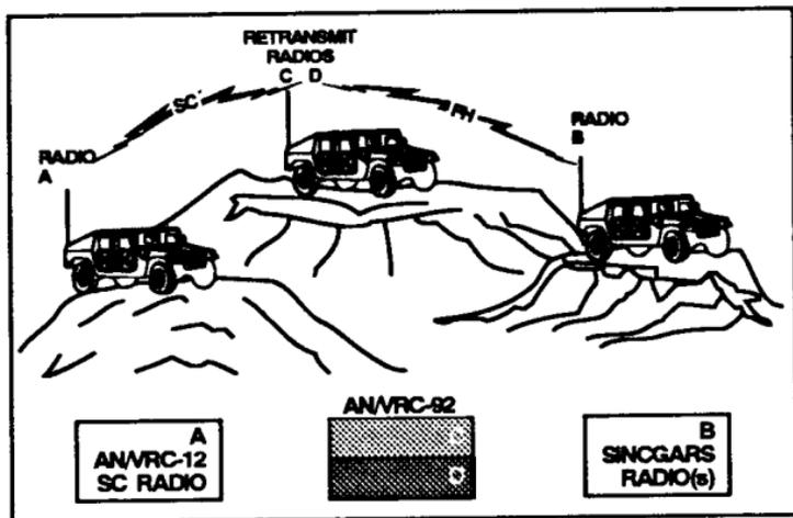
Figure 4-4. SC to FH retransmission operation.
