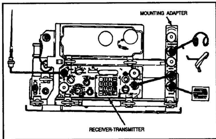
Figure 4-8. Radio sets, AN/VRC-87 and AN/VRC-88.
