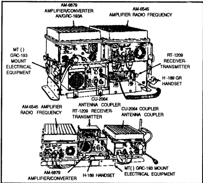
Figure 4-15. Radio set, AN/GRC-193A.
