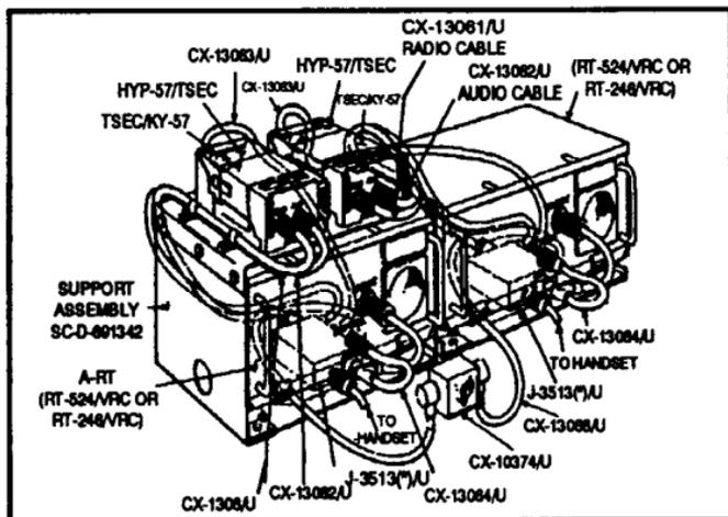
Figure 4-3. Radio set, AN/VRC-49 (secure).
