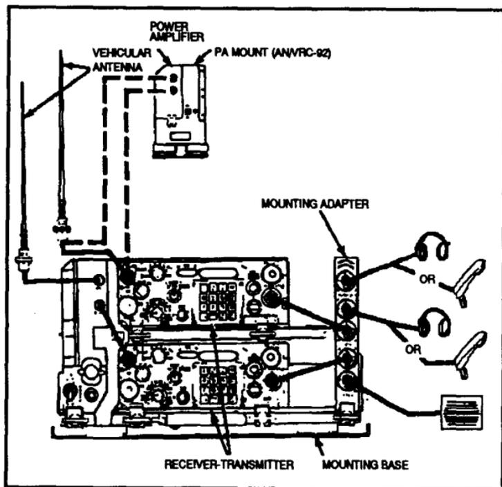
*Figure 4-10. Radio sets, AN/VRC-89, AN/VRC-91, and AN/VRC-92.*
