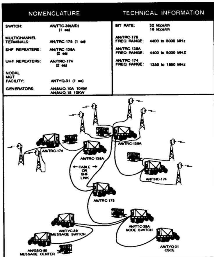
Figure 3-26. Typical TRI-TAC area node.
