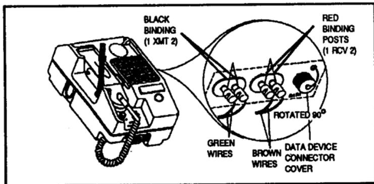
*Figure 3-29. DNVT, TA-1035/U and field wire connections.*
