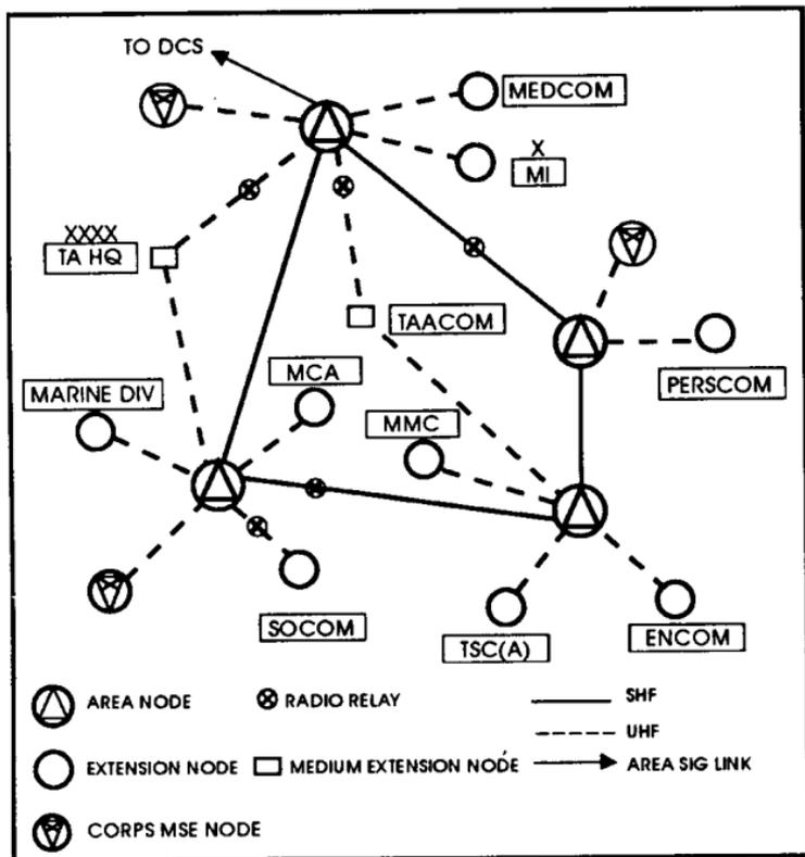
Figure 3-25. TRI-TAC area communications system.
