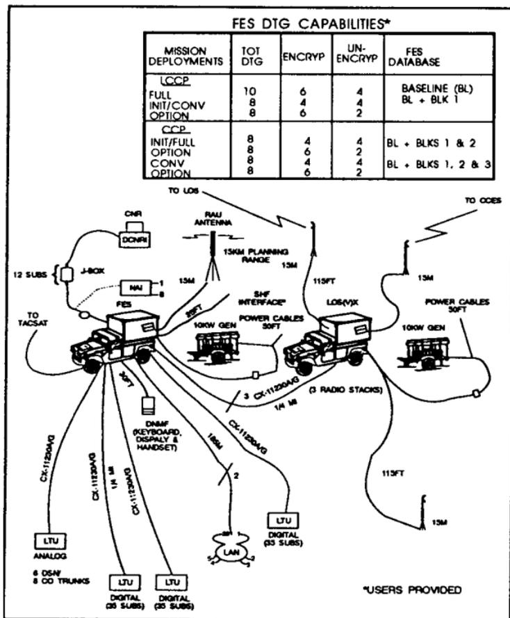
Figure 3-15. Typical CCPS deployment.
