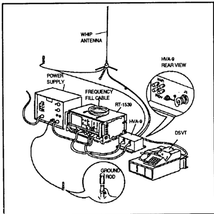
*Figure 3-32. Stand-alone kit (MK-2565/AN/VRC-97) with MSRT.*
