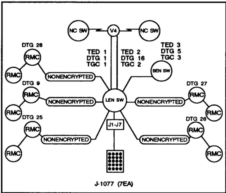
Figure 3-21. LEN switch DTG/TGC standard database.
