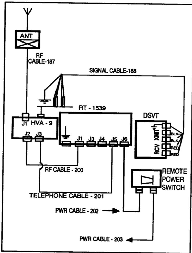
Figure 3-33. MSRT wiring diagram.
