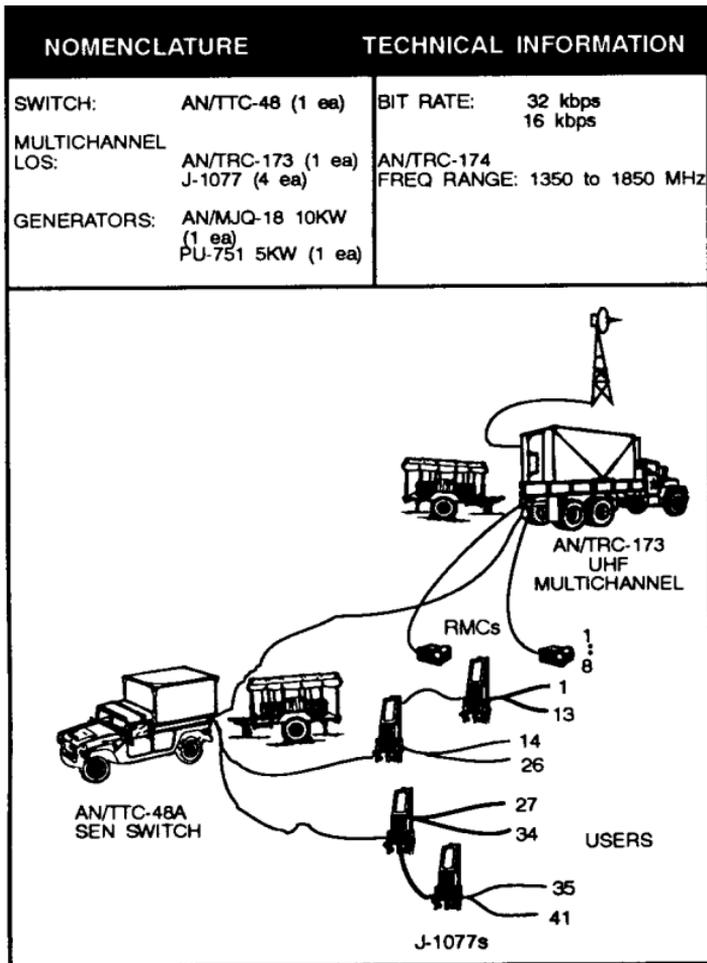
Figure 3-27. Typical TRI-TAC extension node.
