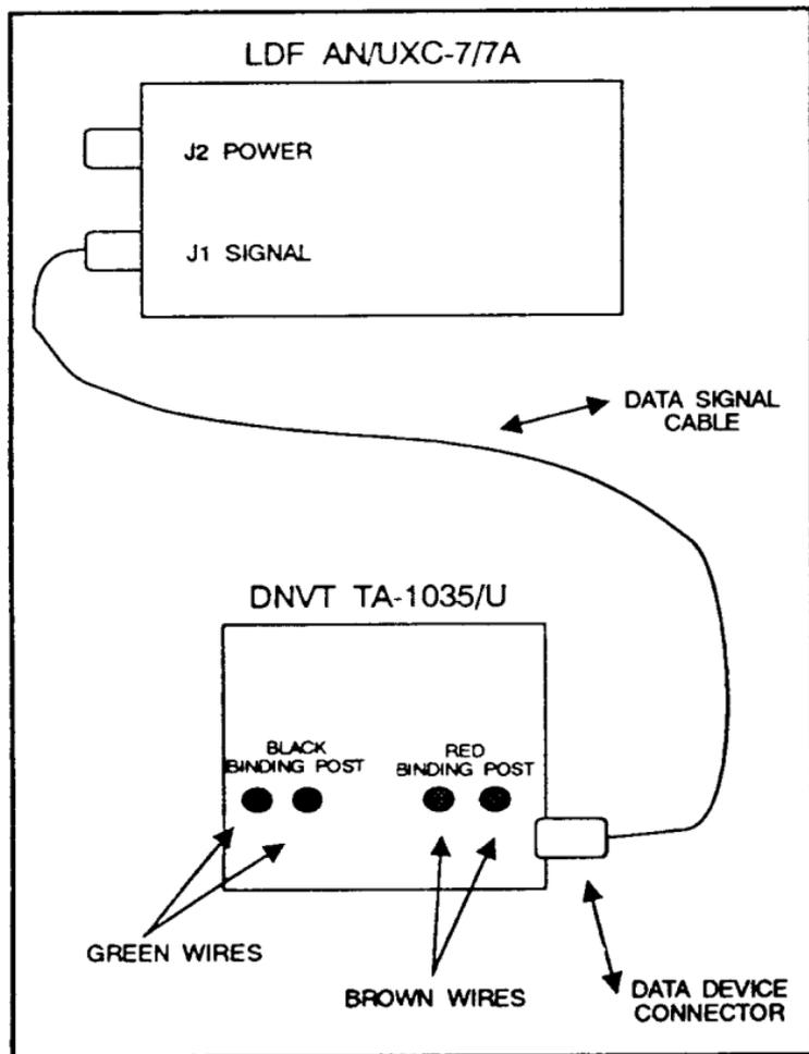
Figure 3-38. MSE telephone interface to LDF.
