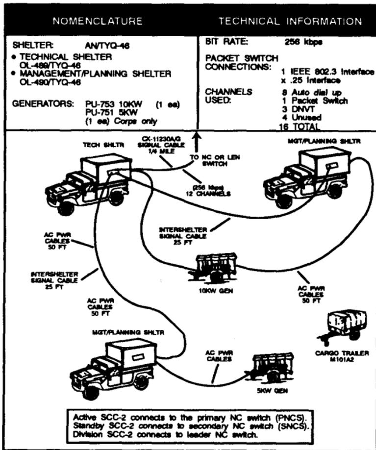
Figure 3-10. Typical corps SCC-2 configuration.
