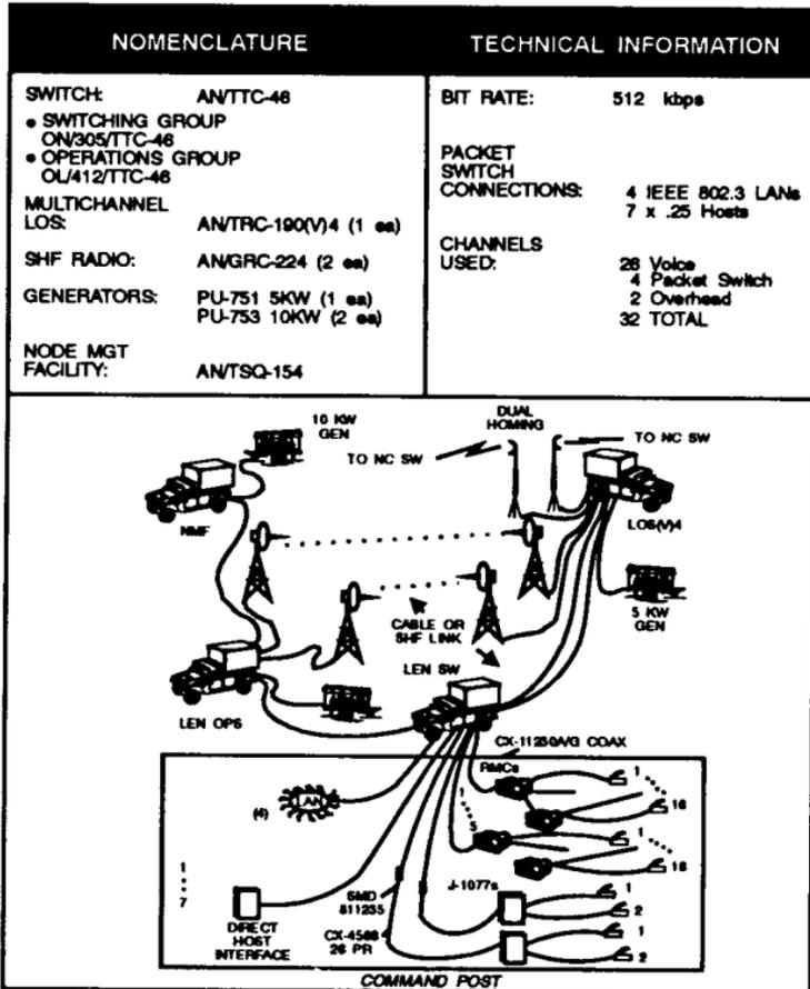
Figure 3-6. Typical LENO configuration.
