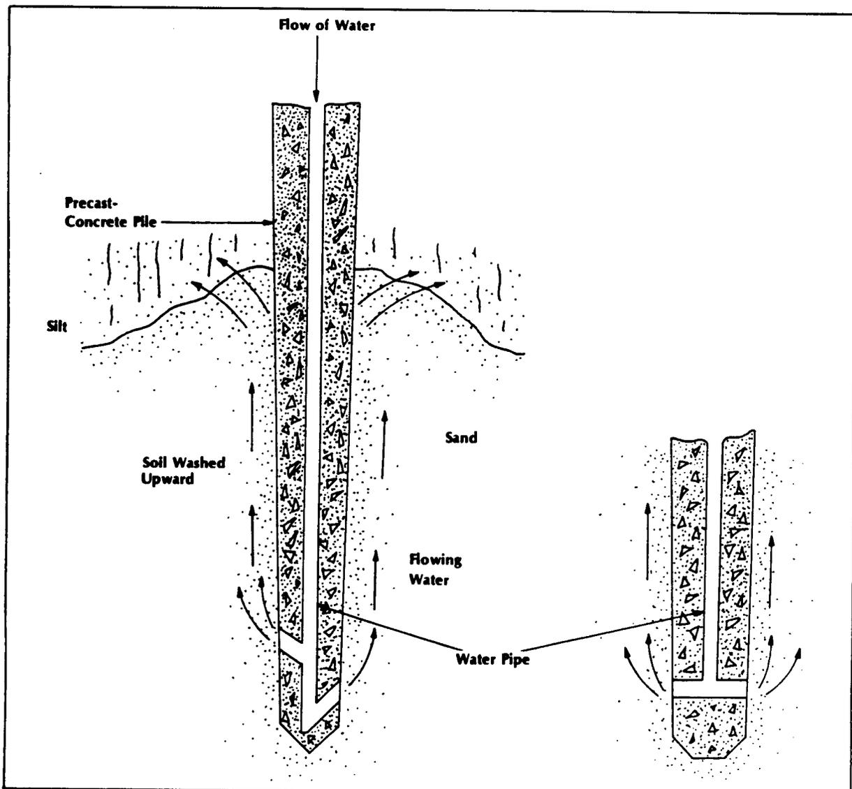
Figure 4-15 Precast concrete piles with internal jetting pipes
