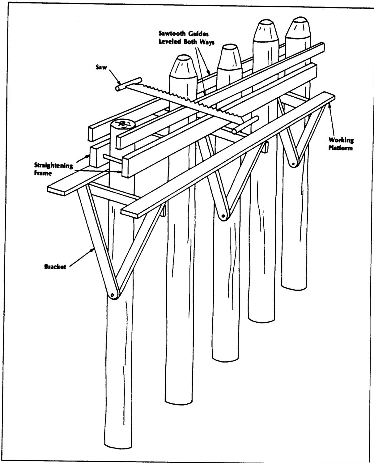
Figure 4-23 Cutting timber pile bent to final height
