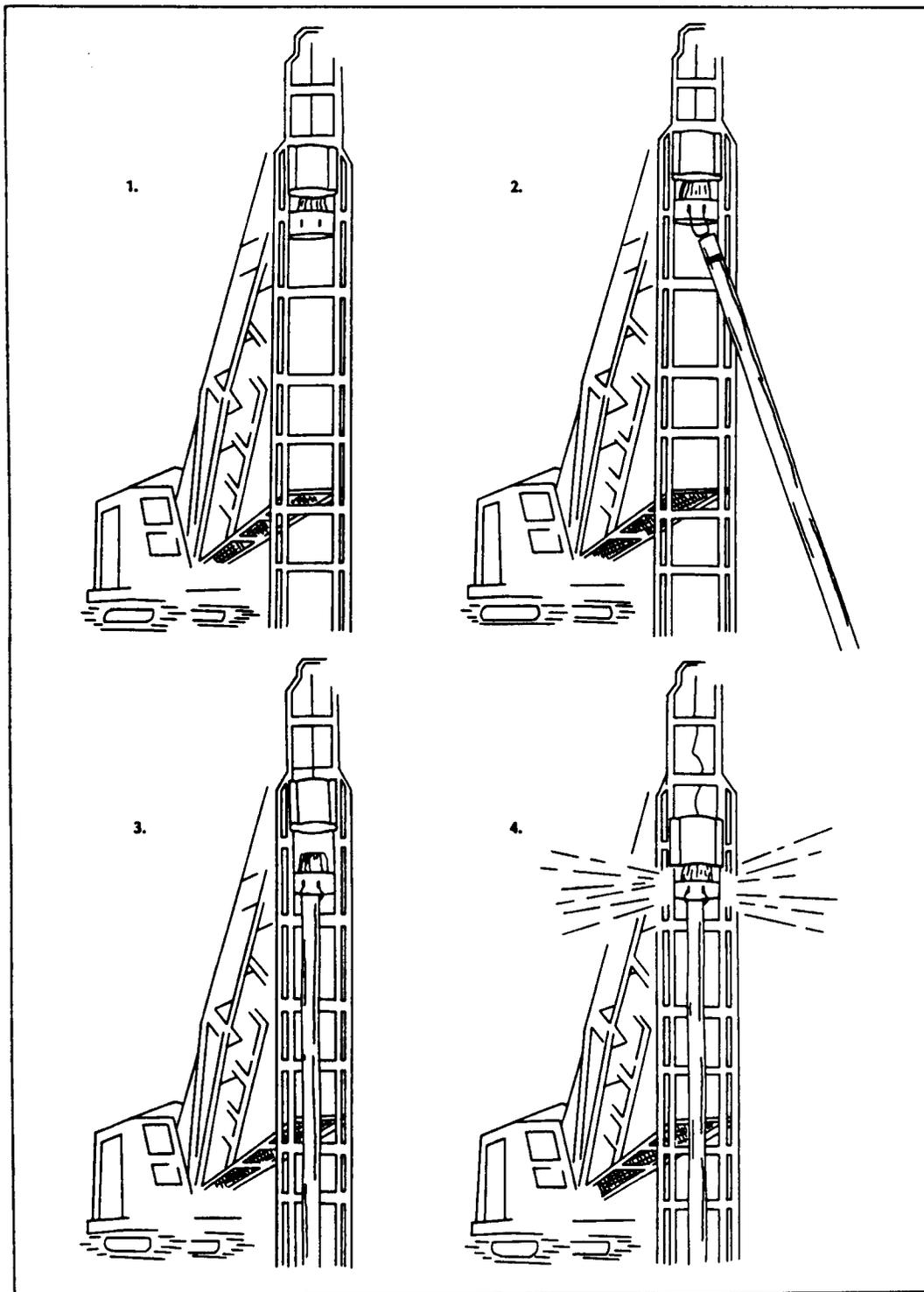
Figure 4-7 Basic steps in setting and driving piles
