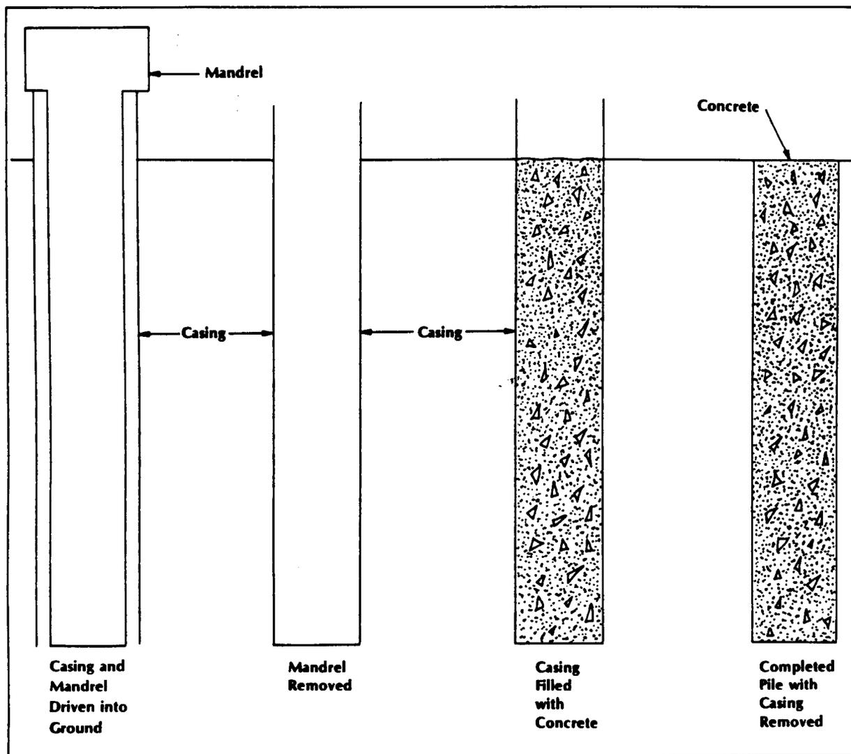
Figure 4-24 Procedure for placing cast-in-ground concrete piles
