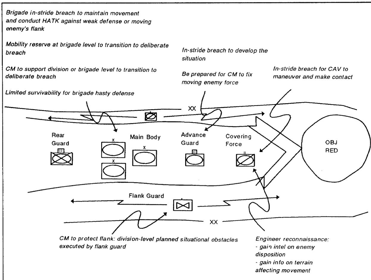
Figure 3-4. Engineer support to a MTC: armored
