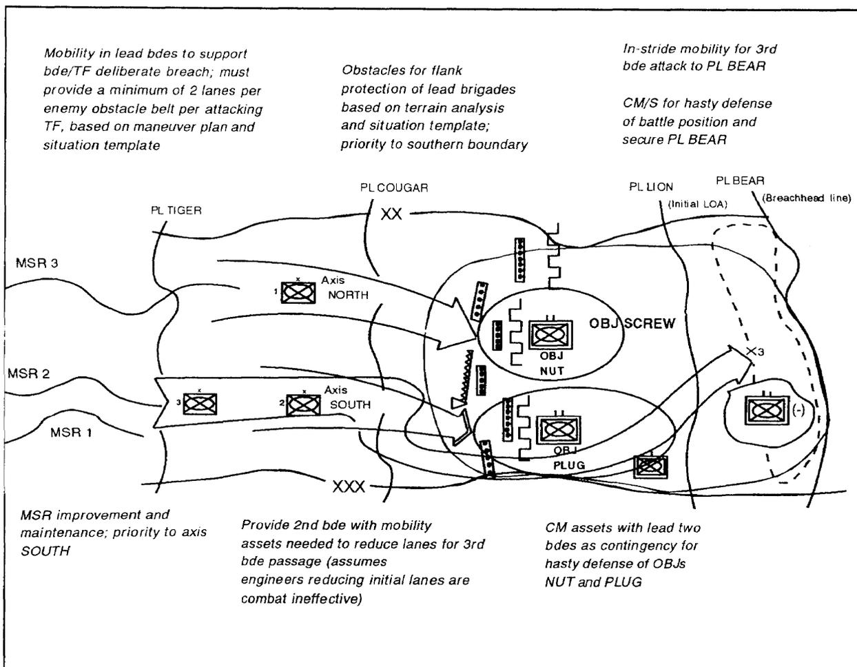
Figure 3-8. Engineer support to a DATK: armored
