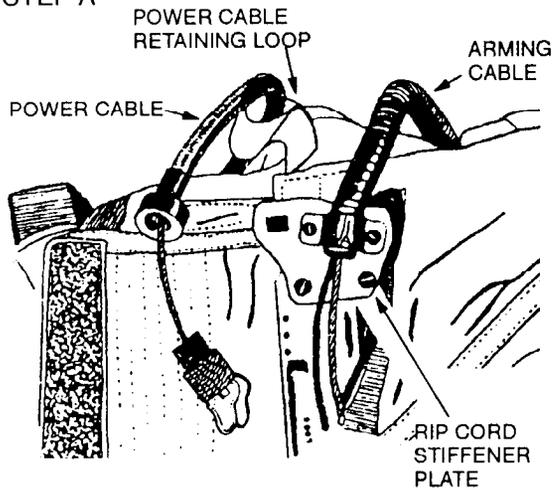
Pass the upper end of the arming cable and housing through the power cable retaining loop at the upper end of the pack, and route it toward the rip cord stiffener plate.
