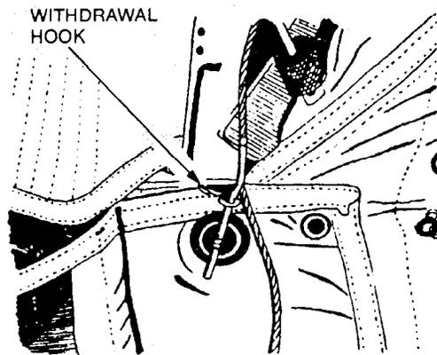
Unscrew the knurled locking nut on the upper end of the power cable and remove the withdrawal hook from the slotted retainers.
