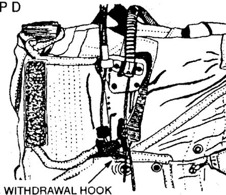
Install the withdrawal hook on the first rip cord locking pin above the first locking cone with the closed, rounded end of the hook under the rip cord cable and against the upper end of the pin. Ensure that the hook does not go around the cable. Reinstall the open end of the hook in the hook retainer slot and secure it to the retainer by screwing the knurled locking nut back across the retainer.
