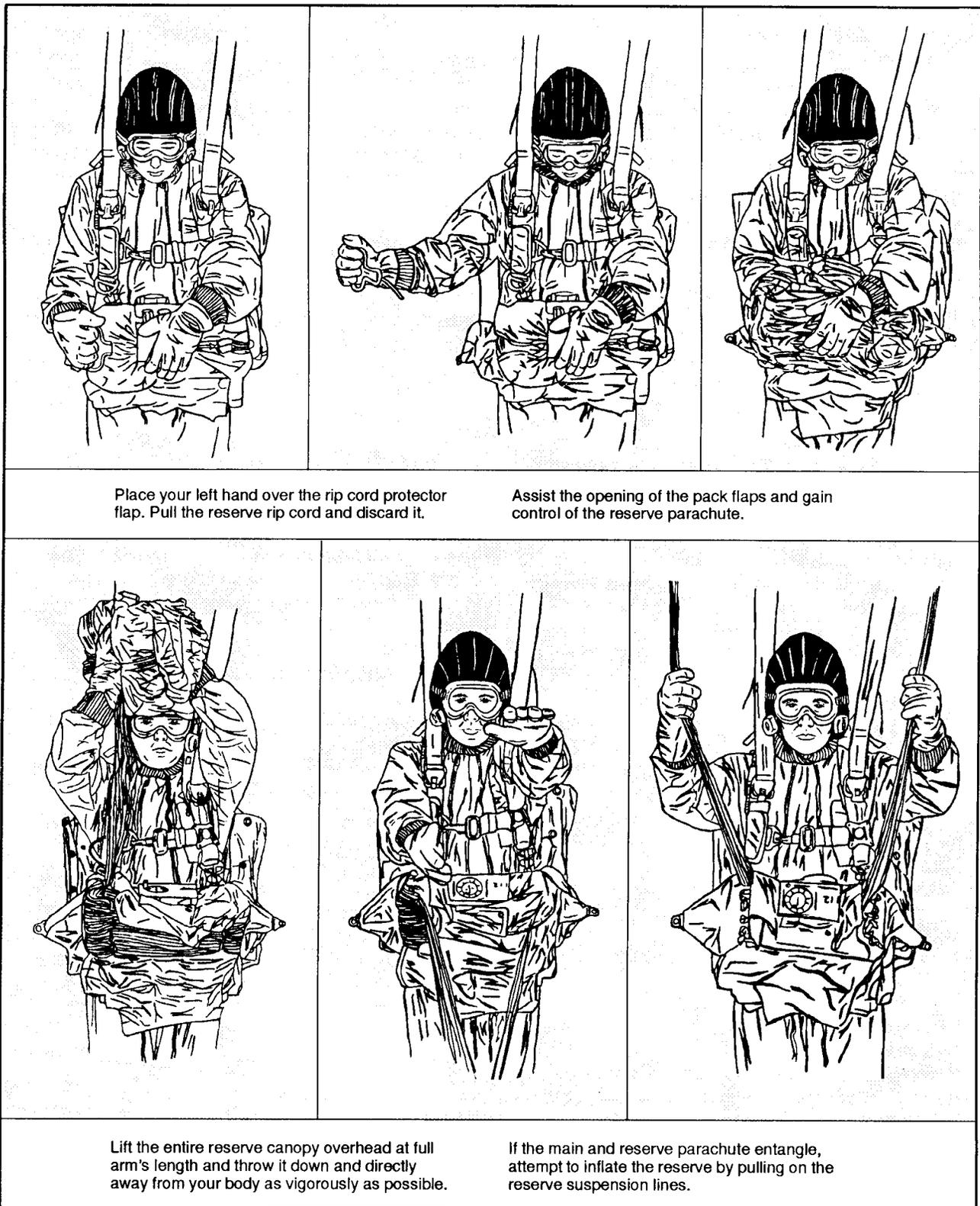
Figure A-10. Controlled method of reserve deployment.
