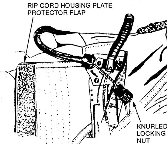
Rotate the power cable housing end 90 degrees clockwise to lock the key in the slot and secure the housing to the plate.
